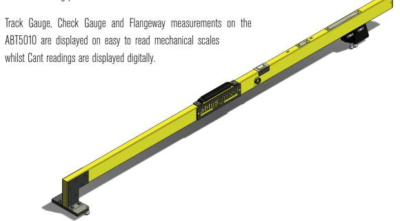
Constructed from hard wearing GRP, the Inspectors Gauge is electrically non-conductive making it suitable for use in areas of 3rd and 4th rail electrification. The ABT5010 is available in both Imperial and Metric versions for multiple track widths.
