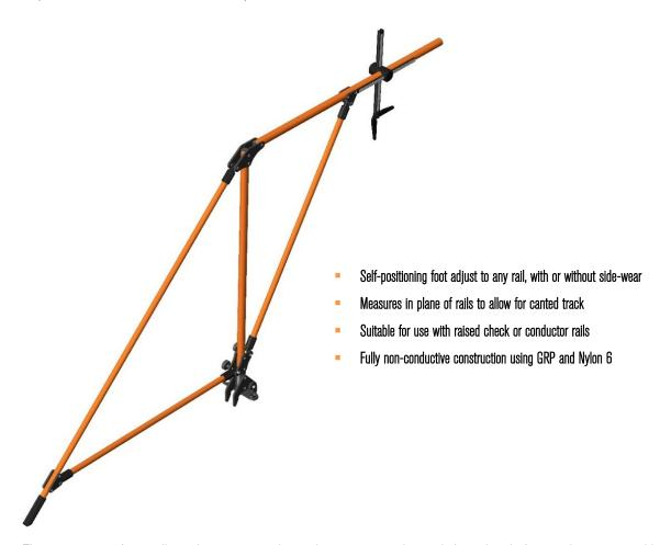
The unique open frame allows the operator to lower the gauge onto the track from the platform and move it quickly in the event of a passing train. Height and offset measurements are made by means of a sprung measurement stick. A self-positioning foot adjusts to any rail type, while the opposite rail is referenced to account the train tilt.
